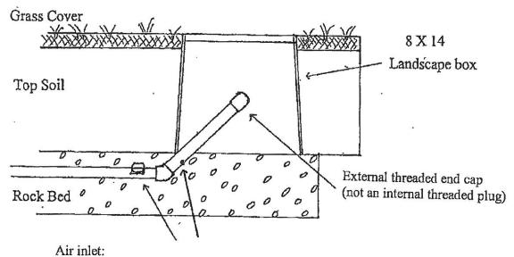
Last perforation is on top of pipe with an orifice shield, or on under-side of upper pipe as shown.
